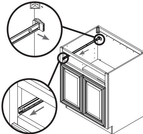
Insert the drawer box. Ensure that the drawer box glide members slide through the plastic guide at the front of the cabinet member on each side.
