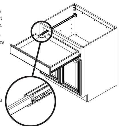
**NOTE:** Drawer should install smoothly but there may be minor resistance when the drawer is approximately half to two-thirds installed. This is normal, and the drawer should push through this smoothly to seat properly.
