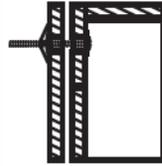
**DRYWALL:** Drill holes and secure to the wall with toggle bolts.
