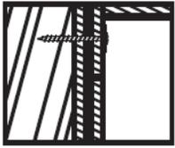
**STUDS:** Secure to wall with #10 x 3" screws at stud location.
