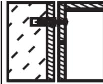
**CONCRETE:** Drill 1/4" holes, insert #10 wall anchors and secure to wall with #10 x 3" screws.
